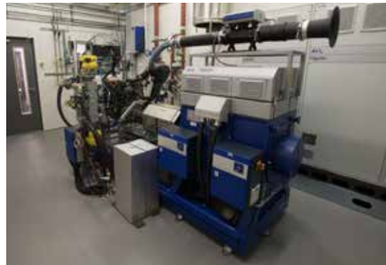
Advanced powertrain dynamic control and calibration test facility
